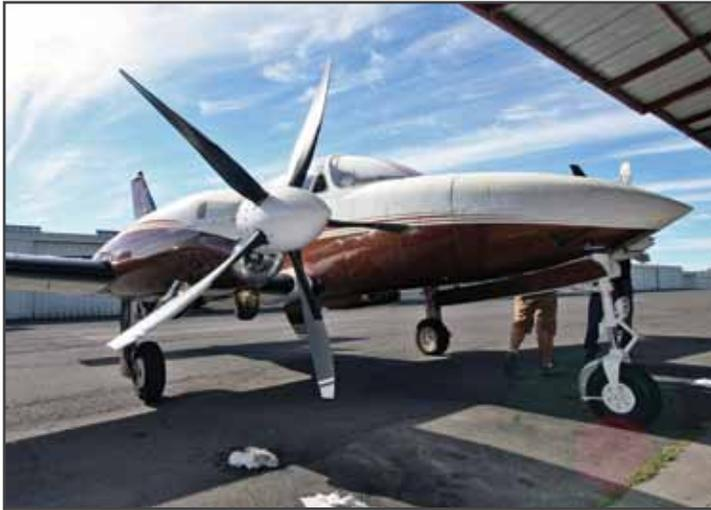
Experimentation continues on the 340 turbine Silver Eagle. Here's one installed with five-bladed composite props. Phenominal climb rates of 3,500 fpm or higher are available. Naturally, most pilots prefer lower rates that allow them to see over the nose, but the performance is there if needed. For more information visit O&N's website at [www.onaircraft.com](http://www.onaircraft.com).
